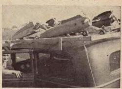
The family car can be quickly converted into a model airplane trailer by the method shown above. A pine frame covered with chicken wire is tied to the car top to carry the planes. Be sure to put padding under the frame to prevent scratching the top.
