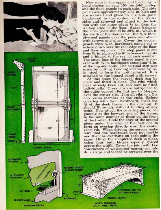
joint. Spread calking compound under the first strip and fold the edges of both strips as they are tacked. Do not use glue as it may be necessary to renew the canvas covering after several seasons of service.
