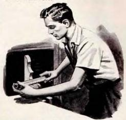
When sanding the edge of an inside curve or circle, the work goes much faster and easier if the sandpaper is wrapped around a piece of pipe about 6 in. long. The diameter of the pipe will depend on the radius of the curve to be sanded. Using the pipe also helps to keep the sandpaper square with the work.
