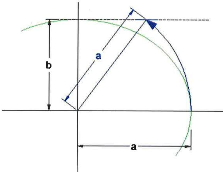
Draw a circle around the centre from the major axis (that is, with a radius equal to 'a') until it reaches a line drawn through the end of the minor axis
