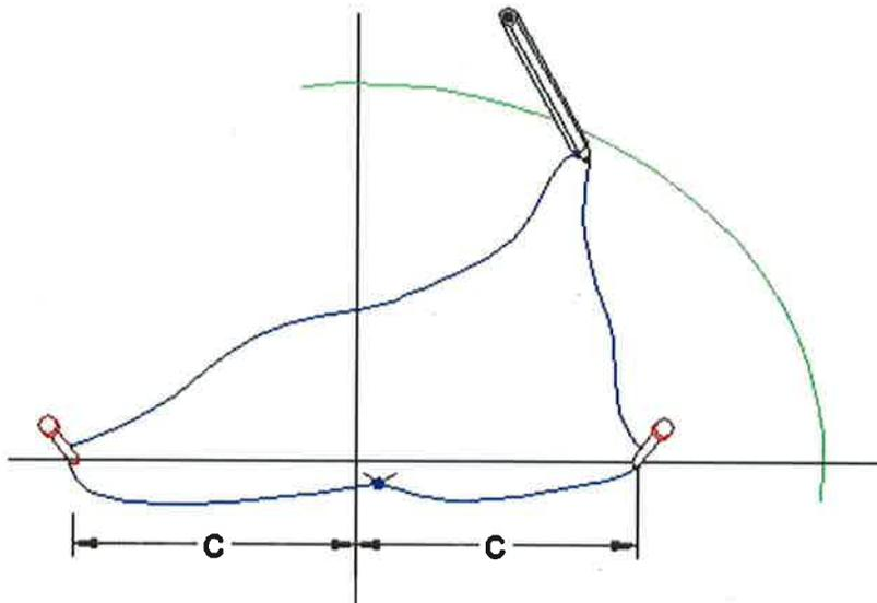
This method is similar to method 1, except the string is not tied to either nail – instead it passes around both nails and the two ends are tied together.
