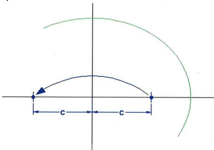
Locate the second focus by going the same distance 'c' on the other side of the minor axis.
